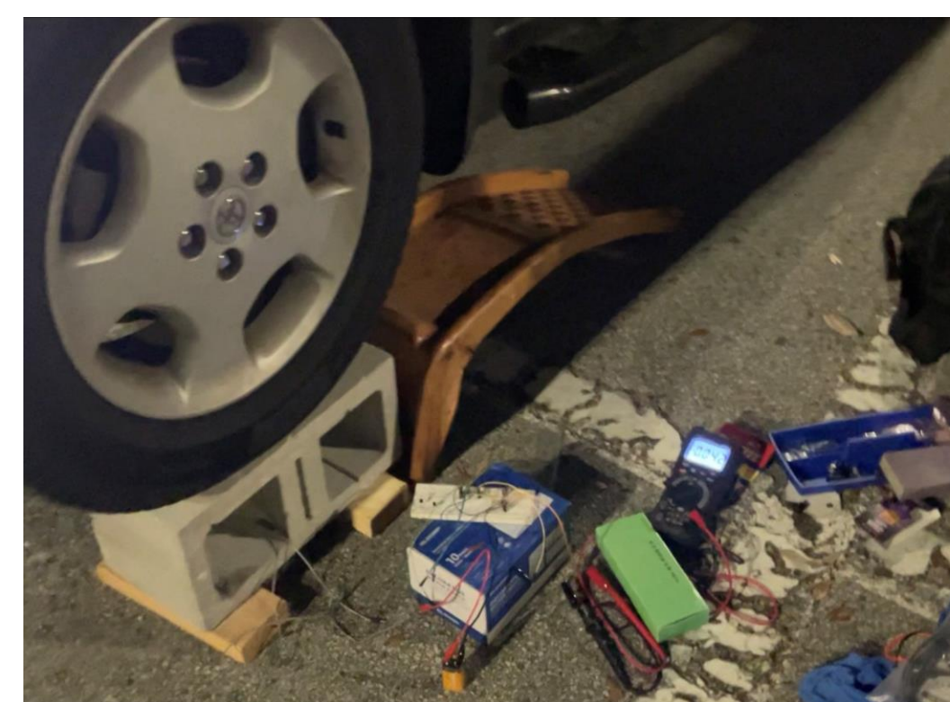
Figure 4. Wheatstone Bridge Validation Test
